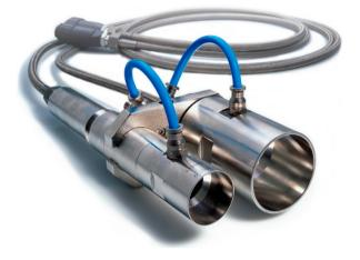
RTS-211 is an optical felt speed triggering sensor for paper machine runnability monitoring. It detects the press felt trade line by measuring the intensity of reflected light and generates a pulse for each felt revolution. Pulse signal can be used in synchronized vibration measurements and to calculate felt length in press section runnability analysis applications.
