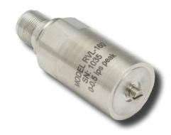
RVL-160 is a true RMS velocity output sensor for mechanical condition monitoring. It is typically used for continuous overall vibration level monitoring in industrial control systems. The sensor provides a 4-20 mA output and can therefore be easily connected to any PLC or DCS.
