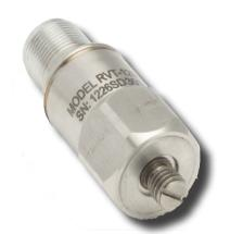
RVT-135 is a high quality industrial accelerometer for mechanical condition monitoring. It has extended low end frequency response for monitoring of slow turning machinery. It can be used with on-line systems as well as portable data collectors.
