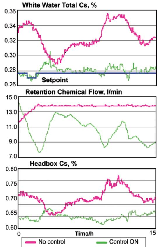
Fig. 2. Wet end consistencies, no control & control on.
