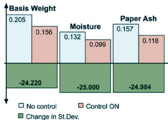
Fig. 3. Effect of control on quality measurement results from the dry end.
