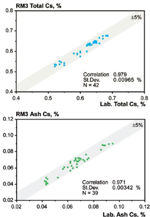
Fig. 1. Valmet RM3 headbox consistency measurements on LWC paper machine.
