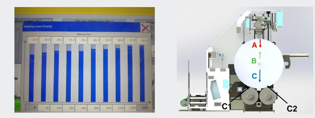
In conventional Hydraulic Rewinders the rider roll linear load (A) and chucks relieving action (B) are actuated by hydraulic cylinders follow pre-established curves, based on the practical operators experience. There Is NO NIP CONTROL and, consequently, NO BULK CONTROL.
