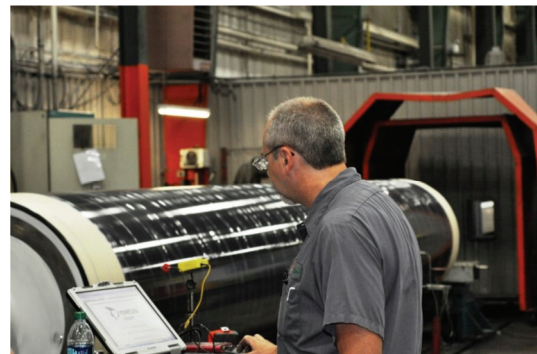
Figure 3: Roll technician performs vibration analysis of a covered roll at Valmet's Columbus, MS roll shop.
