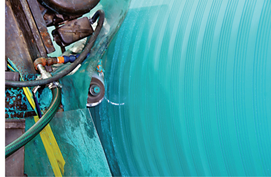
Figure 13: Valmet roll shop manufacturing capabilities include providing roll cover venting solutions for a variety of paper machine applications. In this example the Aiken Service Center is grooving a soft covered winder roll with Valmet's Zatone roll cover.
