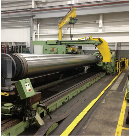
Figure 2: Advanced profile measurement requires specialized dedicated equipment. This Waldrich Siegen grinder equipped with 3D measurement controls is located at the Valmet roll shop in Aiken, SC. The 3D profiles are taken before and after grinding rolls to verify shape, roundness and concentricity.
