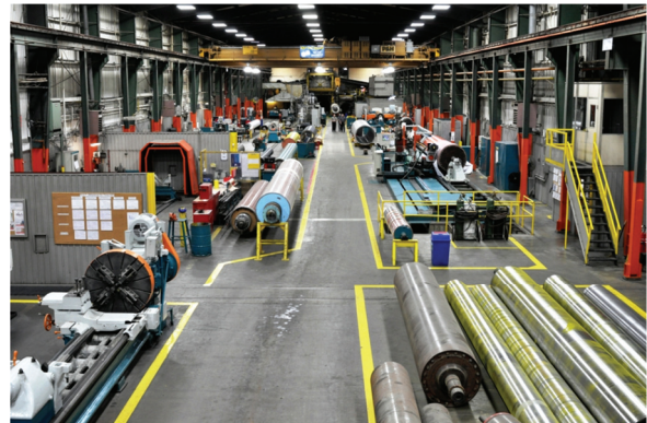
Figure 16: Dozens of rolls are in the process of being recovered, ground and balanced at the Valmet Service Center in Columbus, MS.
