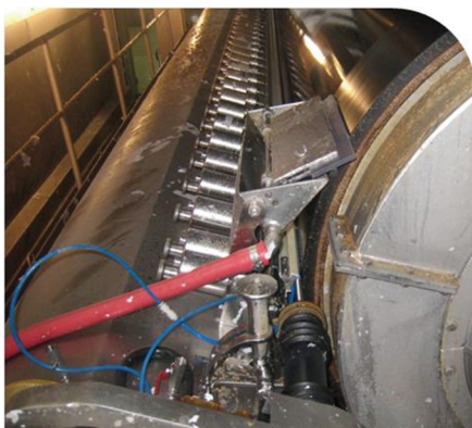
Figure 24. Size press using new two-part rod bed insert improved cost-effectiveness.
