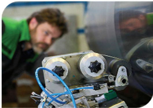
Figure 9. Grinding of the backing roll eliminates runout.
