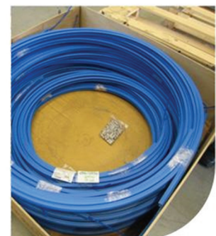
Figure 23. Polyethylene rod bed inserts can be coiled for shipping.
