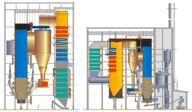
Figure 7. Left: Porin Prosessivoima 60 MWe waste co-firing CFB. Right: Langerbrugge 40 MWe waste-fired CFB boiler.
