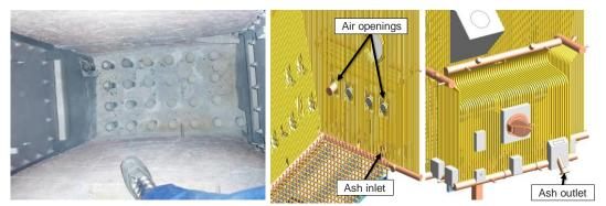
Figure 12. Left: One of the BAC cells. Middle: BAC air and ash connections as seen from the furnace. Right: the BAC from the outside.
