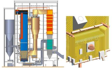
*Figure 6. Left: Manitowoc 60 MWe petcoke-fired CFB boiler. Right: integrated bed ash cooler.*
