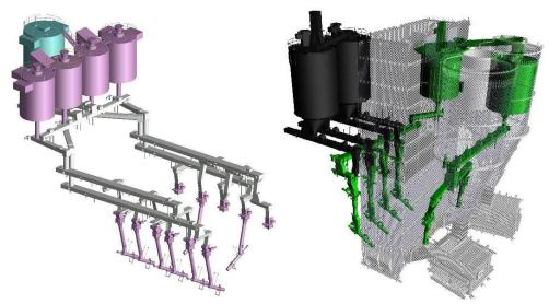
Figure 10. Left: fuel feeding system for 100% coal and 100% biomass case (260 MWe). Right: fuel feeding system for five different fuels (142 MWe).
