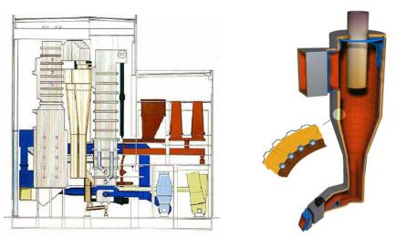
*Figure 3. Left: Örebro 165 MWth CFB boiler with water-cooled cyclone. Start-up: 1990. Fuels: biomass, peat and coal. Right: principle of water-cooled membrane cyclone.*
