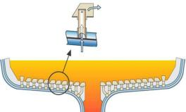
Figure 11. Top: primary air nozzle for biomass. Bottom: primary air nozzle for waste.
