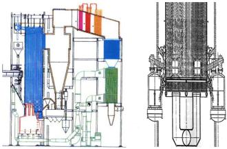
Figure 2. Left: Wheelabrator Frackville Energy Inc., PA, USA CFB boiler. Fuel: culm. Start-up: 1988. Steam values: 51 kg/s, 90 bar, 513 °C. Right: external bed ash cooler design in the 1980s.
