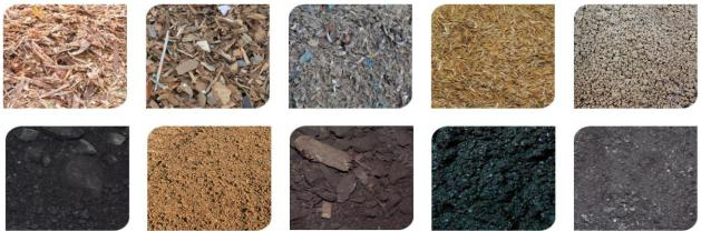
Figure 8. Some fuels used in Valmet CFBs. Top, from left: wood biomass, recycled wood, RDF, agro-biomass, and sludge. Below, from left: bituminous coal, peat, lignite, petcoke, high-ash coal (ash >50%).
